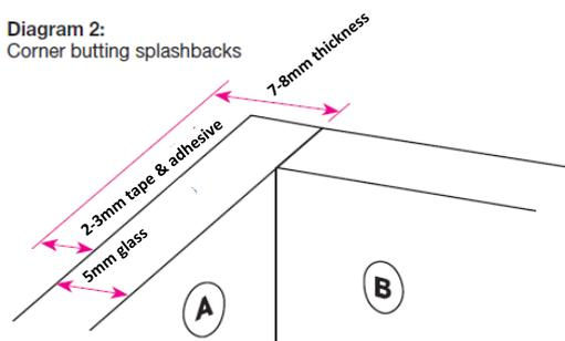
If butting glass pieces together into corners take into account the thickness of your pattern & the glass. Measuring the 2<sup>nd</sup> overlapping piece allow for glass, tape & adhesive thickness. Subtract 7-8mm.
